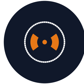
Schematic of the fiber geometry showing the bow-tie configured stress elements and the step index core.
