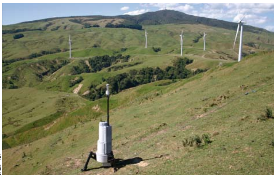
ZephIR is the only realistic alternative to masts for wind farms located in difficult terrain (left). The system consists of three portable pods weighing a total of 150 kg and standing 1.5 m tall (above).
