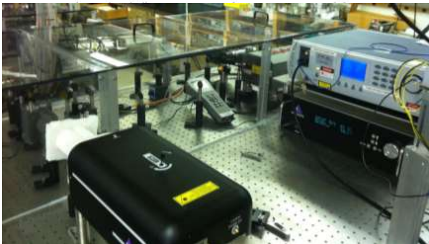
OPO module, controller and IPG fiber amplifier
